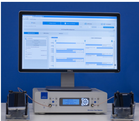
Wireless Test Station with two devices under test
